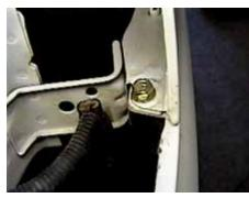
**3.** Just under headlight assembly, remove one push pin on fascia, both sides. Remove one metric bolt behind assembly with the 10MM socket, both sides.
