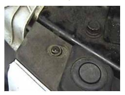
**1.** Remove the six push pins and six phillips head screws from black plastic on the top side of fascia and set aside.
