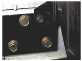
**10.** Align baseplate with tie down bracket holes and tighten existing metric bolts using the 13MM socket. Install metric bolts for windshield washer reservoir and air baffle. Note that the brass colored metric bolt goes to the passenger's side. Be sure and use loctite on all bolts before tightening. Tighten according to torque chart in the General Instructions Sheet.
